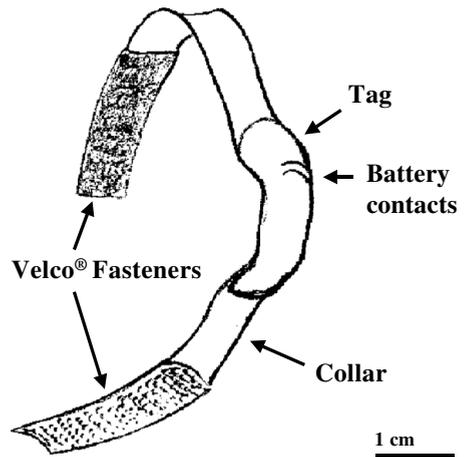
Figure 1. Radio collar for European sousliks (simplified representation).
